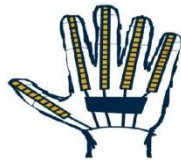
Figure 8. Fixed Flex Sensors on Gloves
