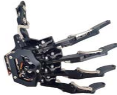
Figure 25. 5 DOF Robotic Hand.
