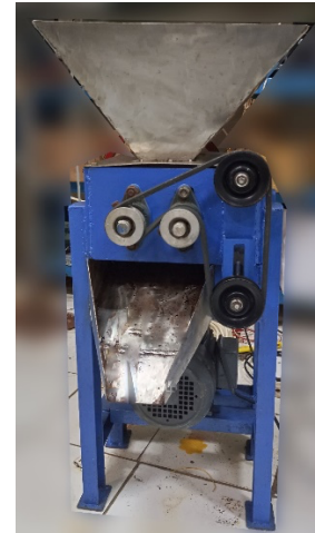
Figure 3. Reversing open belt drive pulleys on a salt crusher machine
